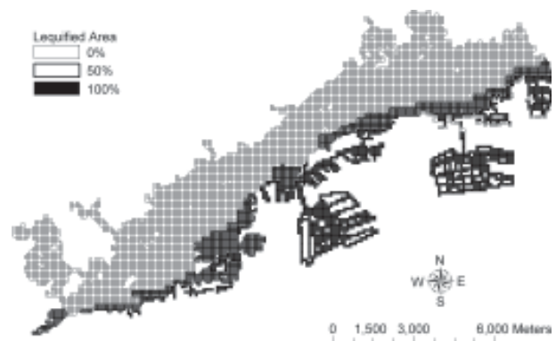
Figure 6. Classification of target mesh due to liquefied area.
