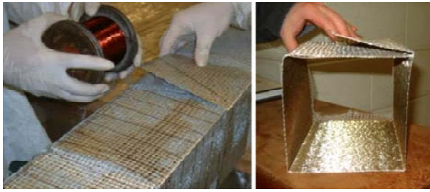
Figure 43. Square of steel reinforced polymer strip and the wire wraps used to apply steel reinforced polymer (Carriere et al., 2009).
