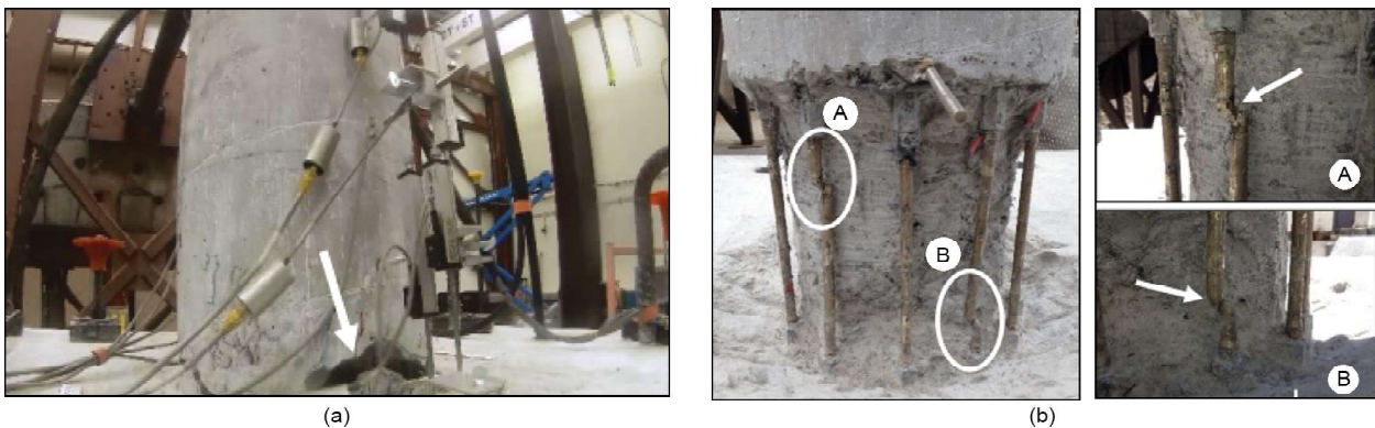
Figure 2. (a) Cracking pattern at the bottom plastic hinge zone during runs 7 and (b) Ruptured SMA bars (Varela & Saïdii, 2014).
