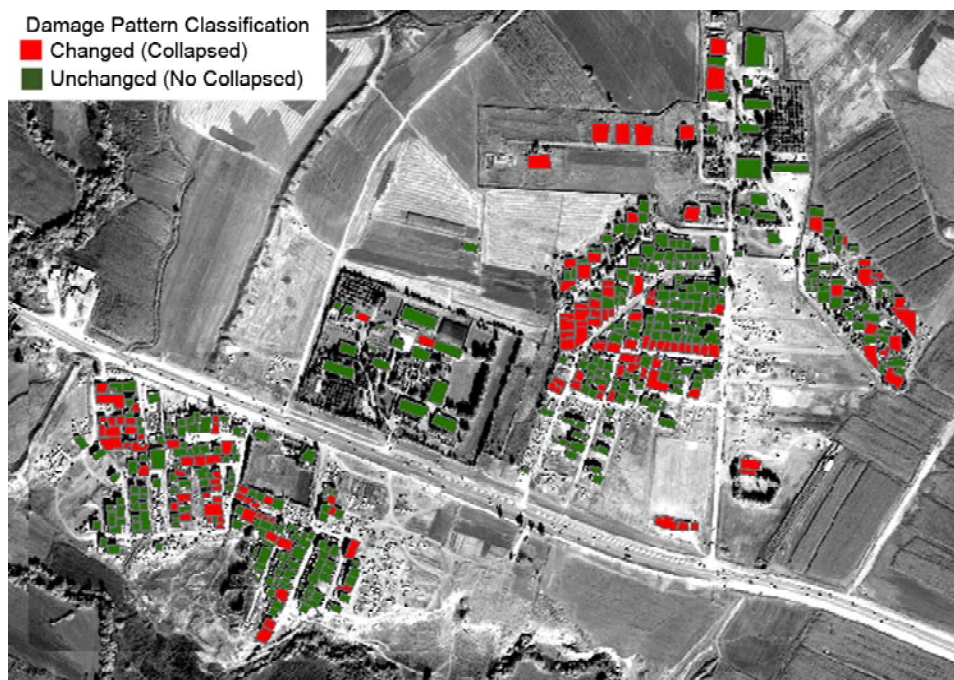
Figure 6. Reference damage map according to the visual interpretation of post-earthquake satellite image.
