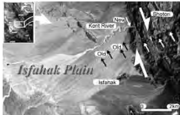
Figure 13. The Landsat TM image shows Korit river south east of Tabas. The river meanders are displaced with a right-lateral strike-slip offset, displacing river courses and alluvium within the Shotori mountains from the north west to south east. The satellite image shows drainage displaced by almost 1.7km at the north west of the south east. The faulting cuts young deposits in beds and continues along the western margin of the Shotori mountains. As it can be seen, a new active front is rising between the Isfahak plain and Shotori mountain, and the existing meanders are in back thrusting with a reverse grade.
