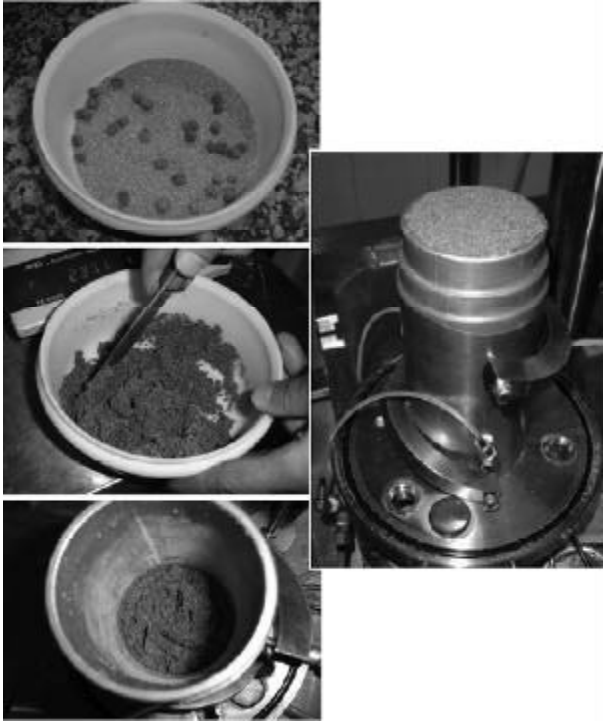
Figure 5. The procedure of preparing the samples.
