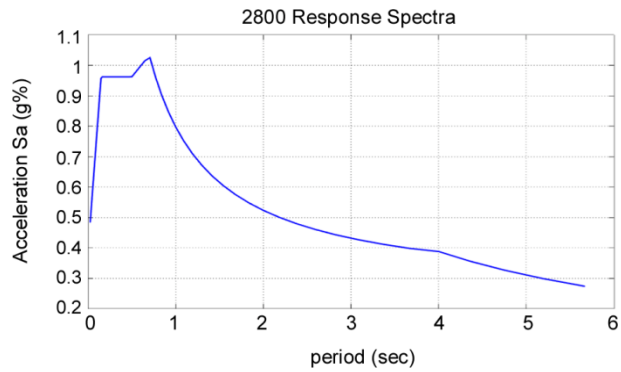
Figure 8. The INBC-zone 1-soil II design spectrum.
