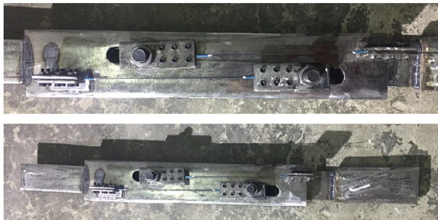
Figure 8. Assembled FD-SMA damper (top).
