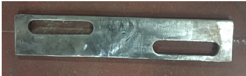
Figure 7. The middle plate of the FD-SMA damper.
