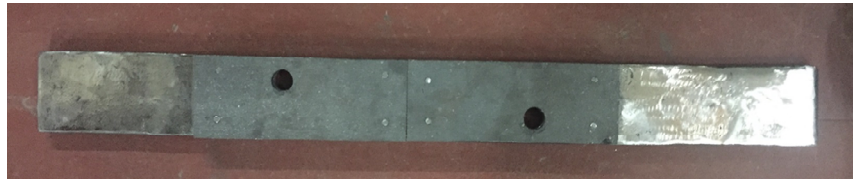
Figure 6. The lower plate of the FD-SMA damper with asbestos 10 mm brake pad.
