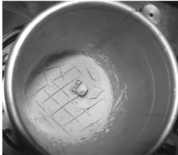
Figure 7. Pure clay specimens for cyclic triaxial test.
