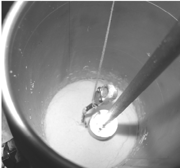
Figure 9. Position of the IPT during compaction of the specimens by tamping hammer.
