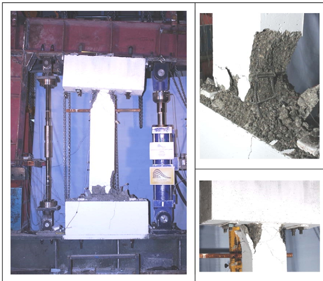
Figure 8. Crack pattern and axial failure in column S3.
