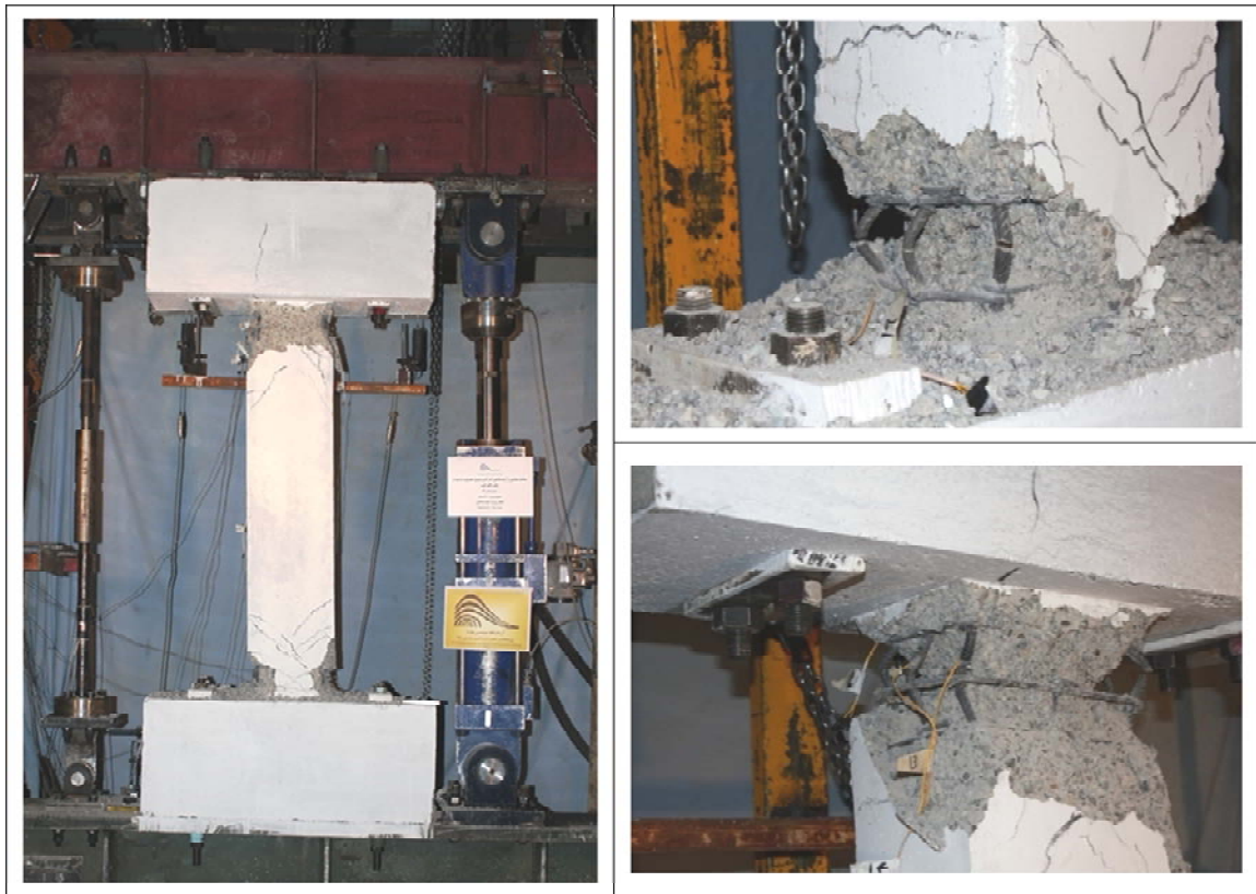
Figure 4. Crack pattern and axial failure in column S1.
