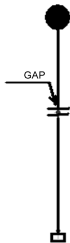
Figure 19. A view of simplified one-degree-of-freedom model.
