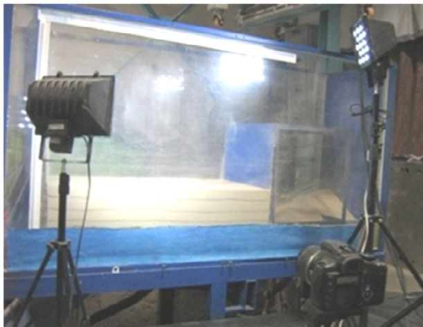
Figure 2. photo of the faulting apparatus (split-box), camera and DC.
