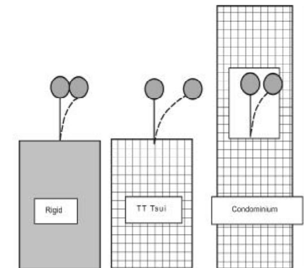
Figure 10. Reduction in floor displacement demand by isolation effects in tall buildings.
