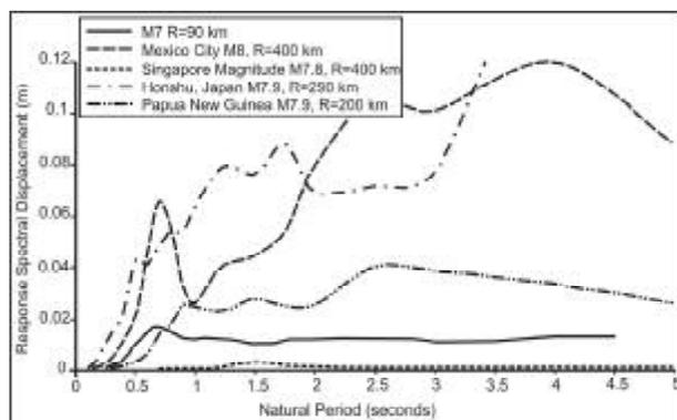
Figure 14. Displacement ground spectra for all accelerograms employed in analyses.
