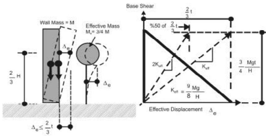
$$\text{Effective Period (100\% disp)} \quad T_{eff} = 2\pi \sqrt{\frac{M_e}{k_{eff}}} = 2\pi \sqrt{\frac{\frac{3}{4}M}{\frac{9 Mg}{8 H}}} = 2\pi \sqrt{\frac{2 H}{3 g}}$$
