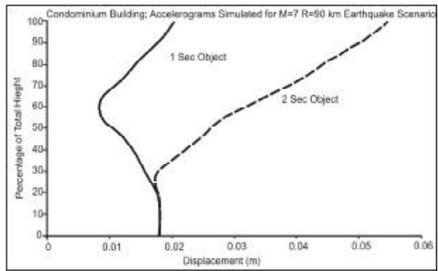
Figure 13. Vertical distribution of floor displacement demand for 1 and 2 sec object floor.
