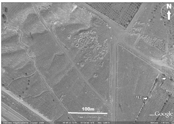
Figure 6. A Quick bird image, Google earth satellite image ( http://www.google earth.com ) of the trench sites, two trenches, TE2 and TE3 in north of Garmdareh (shown in Figure (5)); two lines of wells of ghanat are significant by small cone in west of TE2 . GPS coordinates below the image are corresponded to geographical location of the white flag in south of the trench TE2 .
