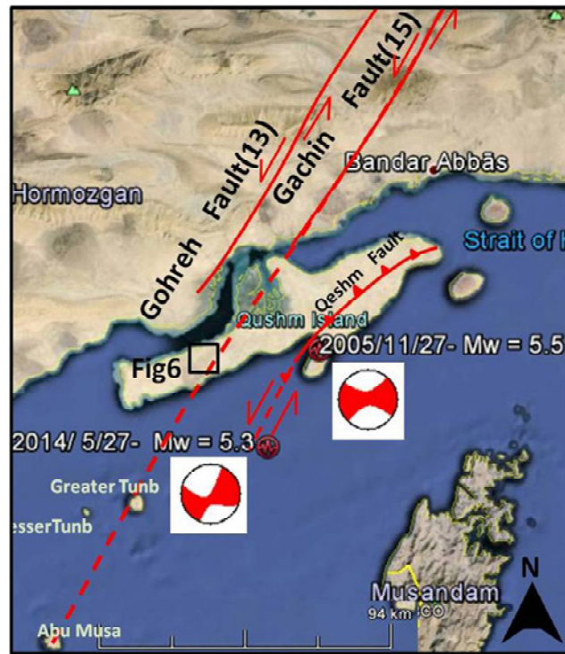
Figure 5. The satellite image of the study area shows Gachin and Qeshm faults. Location and focal mechanism of 2005/11/27 and 2014/5/27 earthquakes are illustrated. The position of Figure (6) is marked by black rectangle.
