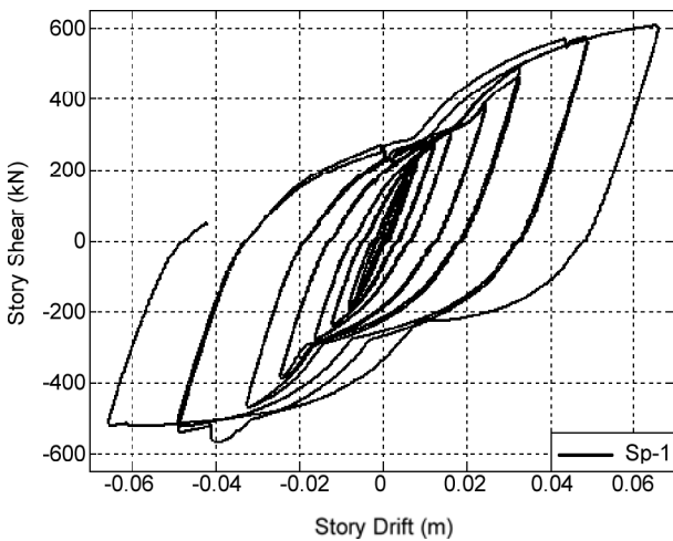
Figure 9. Hysteretic response of specimen SP-1.
