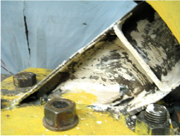
Figure 15. Yielding of the knee at the end of test.
