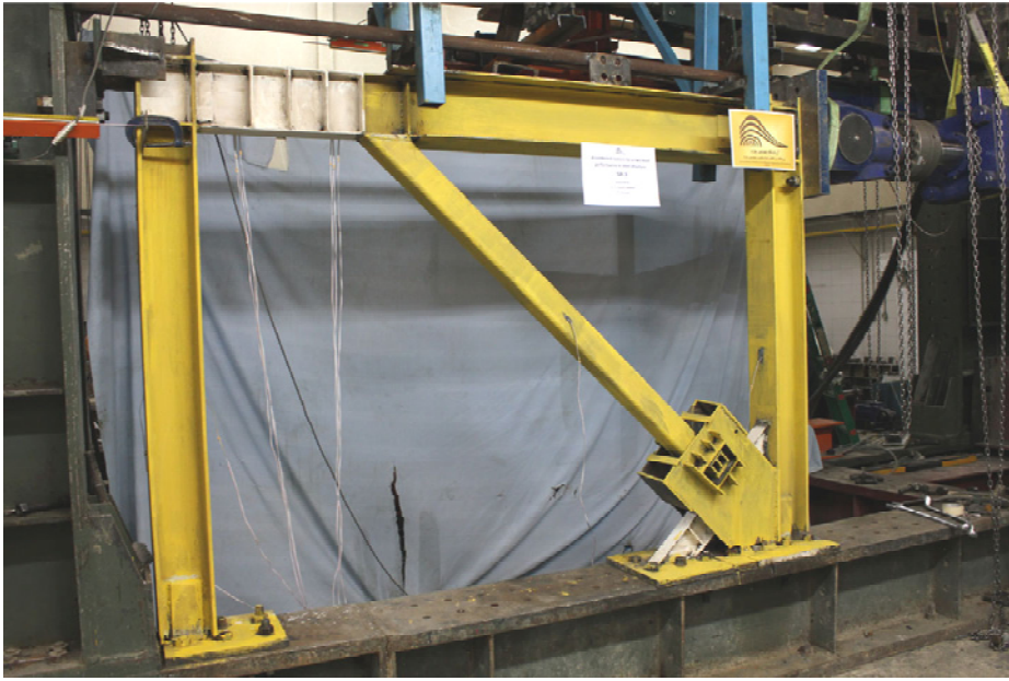
Figure 6. Photograph of EKB frame subassembly.
