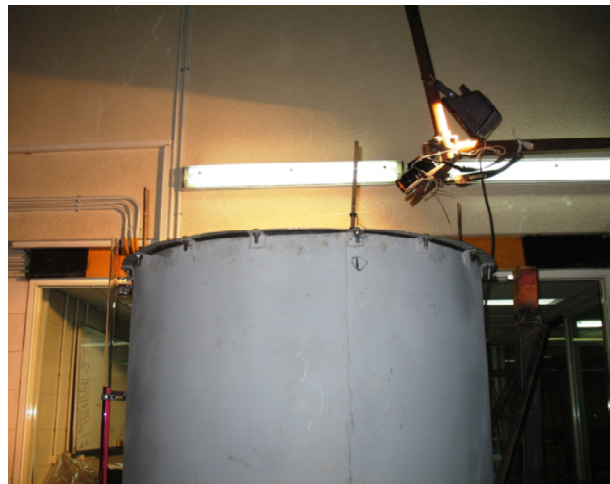
Figure 5. Location of the camera for filming the fluid Sloshing.
