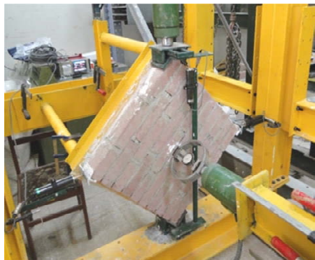
Figure 1. Test set-up for simultaneous application of in-plane and out-of-plane loads.
