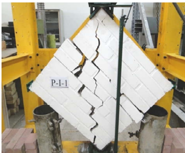
Figure 3. Failure of the wall panels under in-plane shear load.
