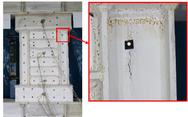
Figure 6. Yielding of the right secondary column web in Sp-1 specimen at 1.5% drift ratio.
