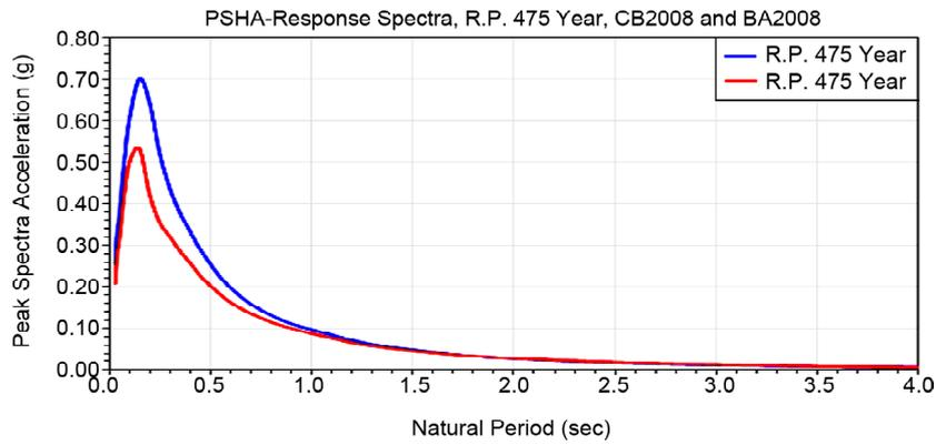
**Figure 2.** Response spectra derived from PSHA method in Bakhtiari dam site with the use of BA2008 & CB2008 attenuation relations, for the R.P. of 475 years.
