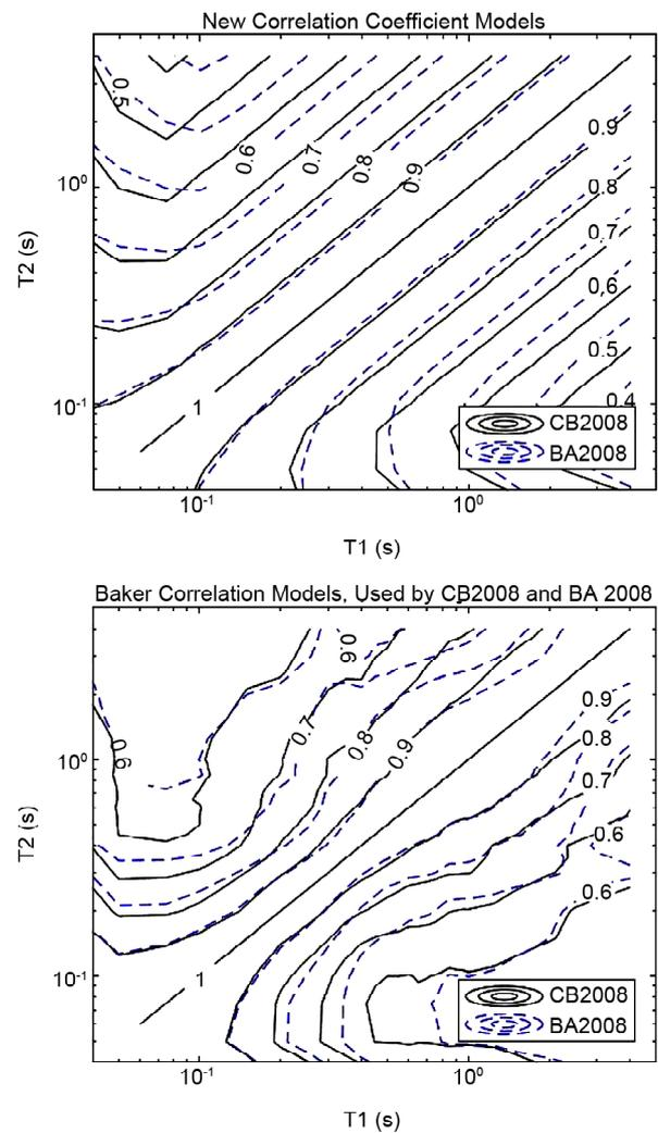
**Figure 7.** Comparison of correlation coefficient curves against  $T_1$  and  $T_2$  periods, before and after correction of fixed coefficients of Baker and Cornell [1] using CB2008 and BA2008 relations, for a set of selected natural ground motions in Zagros region.
