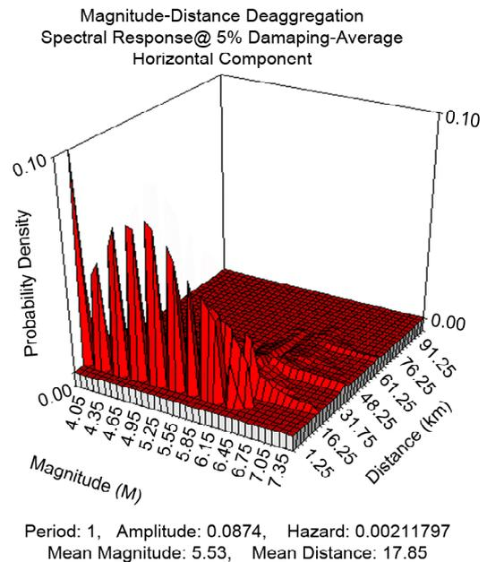
**Figure 3.** Seismic deaggregation by PSHA method in Bakhtiari dam site with the use of CB2008 attenuation relation, for the R.P. of 475 years.
