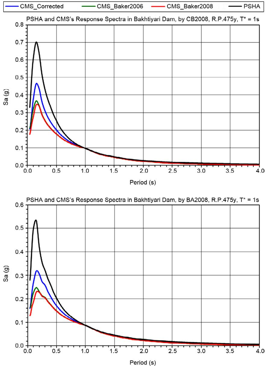
**Figure 8.** Response spectrum of probability seismic hazard analysis (PSHA) and the estimated conditional mean spectra (CMS) for the Bakhtiyari Dam site, based on the Baker and Cornell [1] and Baker and Jayram [2] experimental and modified correlation relationships using the CB2008 & BA2008 attenuation relationship.
