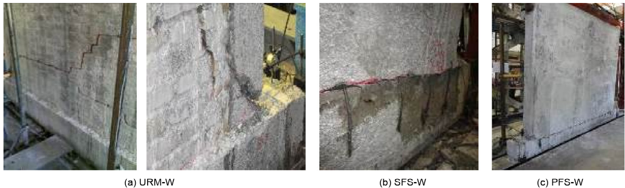
Figure 6. The crack pattern of the walls under cyclic loading.
