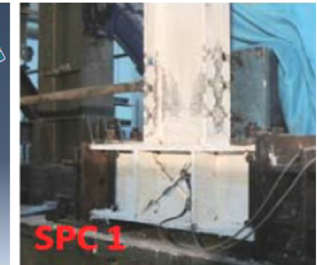
Figure 4. Formation of plastic hinges in experimental and numerical samples.
